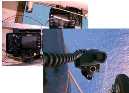
Thermal camera Flir B20HSV
