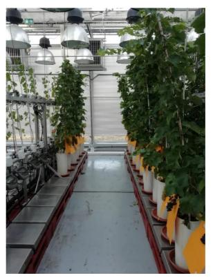
*Fig 3: image of the SupAgro greenhouse. Each plant was positioned on a scale and connected to a self-irrigation system, allowing the weight to be maintained.*
